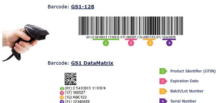
Figure 2. By scanning the GS1 barcode or matrix, important device identifiers are prefilled in the registry
